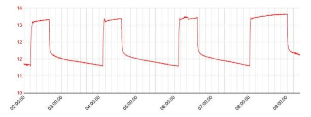
Each rise is caused when the generator turns on, then when the generator turns off, the voltage slowly drops until the generator turns on again.
